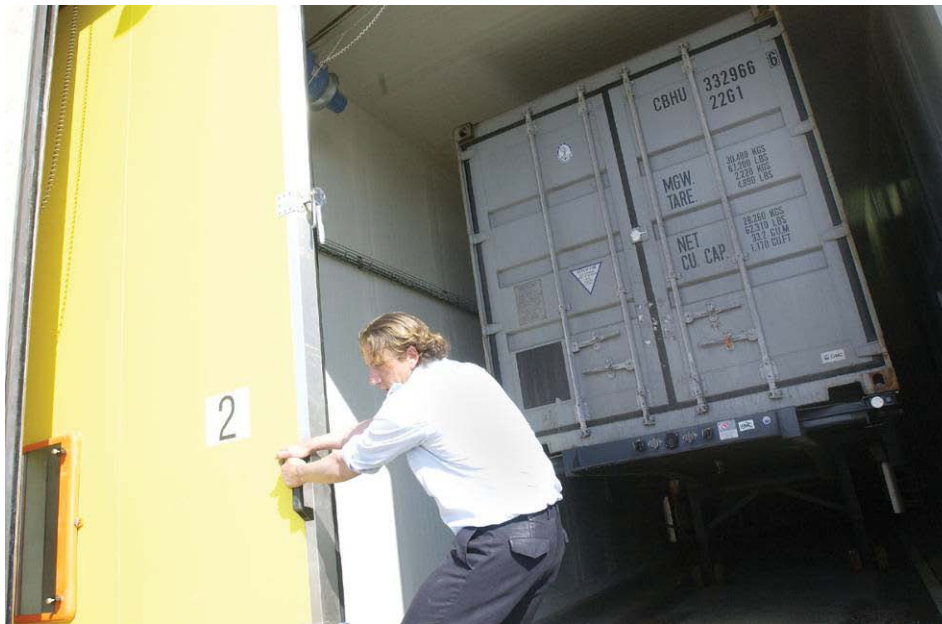
Pict. 2: CA facility which fits 2 TEU in one treatment room
