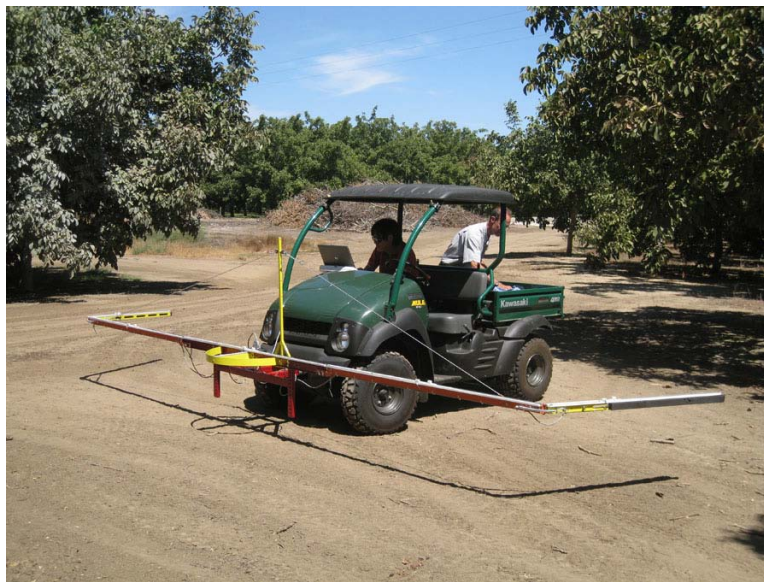
Figure 1. Schematic of the fine-tuned site-specific fumigant application system
